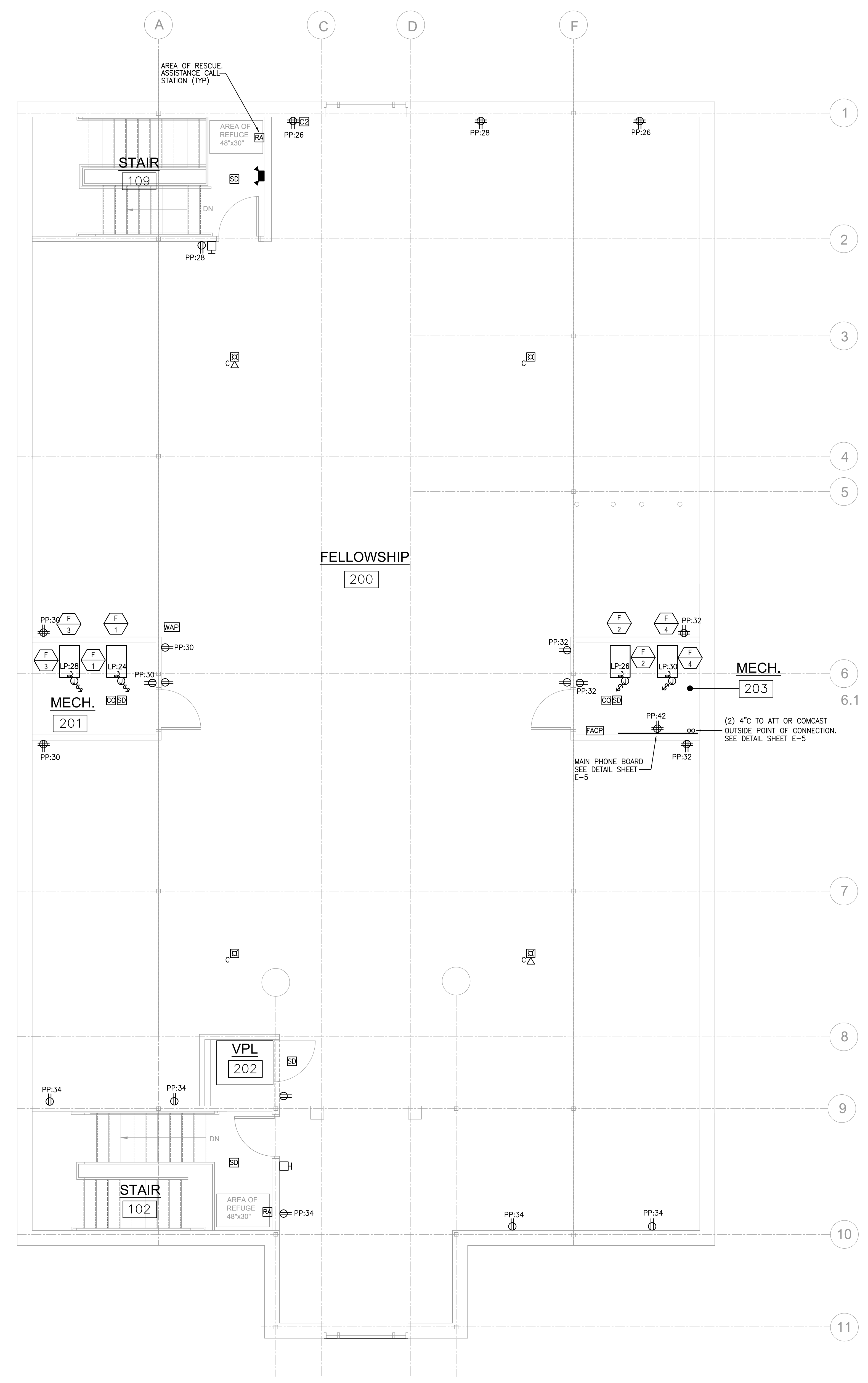
1 SECOND FLOOR PLAN - ELECTRICAL (BASE BID) E-2 SCALE: 1/4" = 1'-0"
